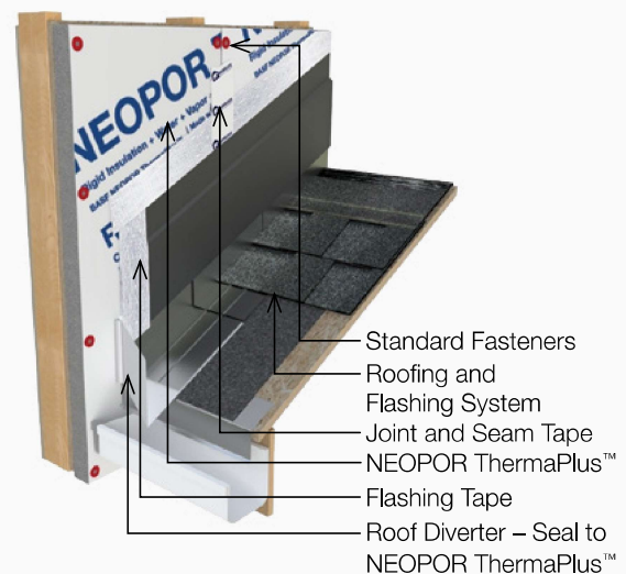
■ Figure 14: Typical Roof Diverter
