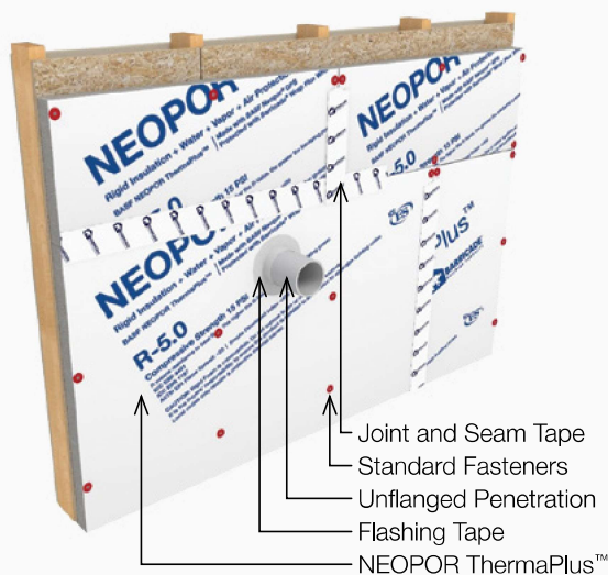
■ Figure 8: Typical Unflanged Penetration (Pipe, etc.)
