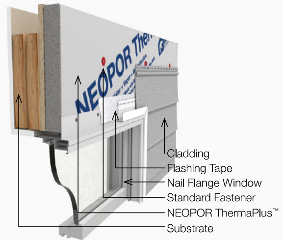
■ Figure 12: Typical Window Head (Jamb Similar) - Nail Flange Window
